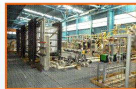
Recovery of wastewater from zinc-plating process for rinse water by EDR process ( China steel company, 700 m<sup>3</sup>/day)
